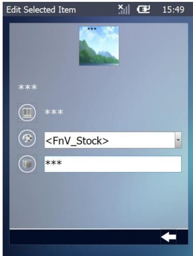
The screen’s editable controls (the “Input Keyboard” and the “Combo Box”) contain a “Variable Assign” and an “Update Record” process. As a result, the selected variable includes the new value and the source data file is also updated.
