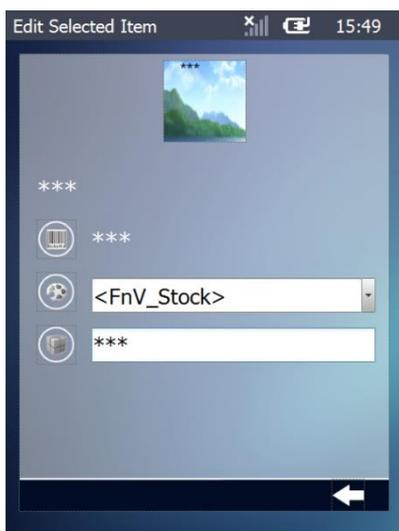
The screen contains “Display Text”, “Display Image”, “Combo Box” and “Input Keyboard” controls. The “Display Text” and “Input Keyboard” controls each display the content of a variable (with specific data file data) and the “Combo Box” displays the value of the selected data file field. One of the “Display Image” controls (“Fruit\_img”) also displays the content of a variable.
